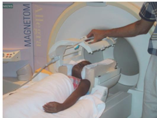
Acoustic noise in the scanning environment is loud, it can reach amplitudes of 113 dB in some magnet environments, but is usually around 90 dB. Although this is well below the U.S. Food and Drug Administration guidelines for acoustic noise levels in an MR system (140 dB), we still require all subjects to wear hearing protection. In the case of children, the headphone system we use reduces the MR noise by 30 dB. This brings the noise down to approximately the level of normal adult conversation.
